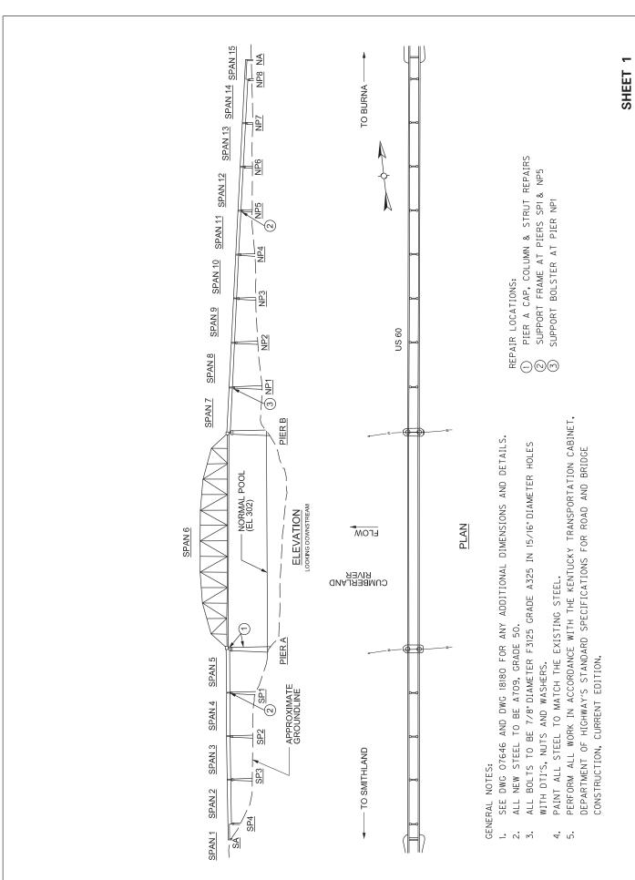
BRIDGE REPAIRS - PLAN AND ELEVATION
