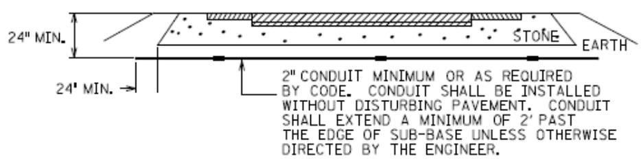
CONDUIT UNDER EXISTING PAVEMENT DETAIL
