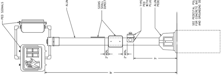
CONTRACTOR SHALL DRILL HOLES IN THE PIPE AND THE TYPE FS BOX NOT EXCEEDING 1/2" IN DIAMETER. CONTRACTOR SHALL USE A ROUND FILE TO REMOVE ALL BURRS AND SHARP EDGES FROM THE HOLES. WIRES SHALL BE PROTECTED WITH HEAT SHRINK TUBING OR VINYL TAPE WHERE THEY PASS THROUGH THE HOLES.
