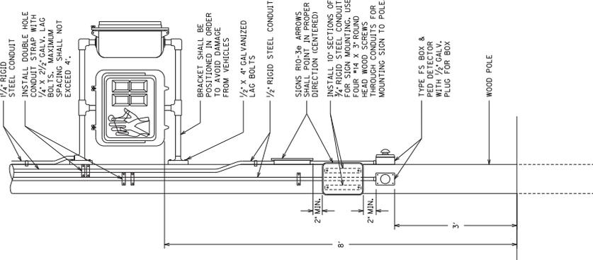
AS A 1/2" PIN HEAD OR ROUND HEAD WOOD SCREWS SHALL BE USED TO SECURE TYPE FS BOX TO WOOD POLE. A MINIMUM OF 2 SCREWS PER BOX, INSTALLED DIAGONALLY, SHALL BE USED.
