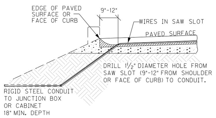
PIEZOELECTRIC SENSOR INSTALLATION
