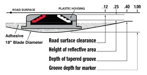
**D. Location and Spacing.** Install the markers in the pattern for high reflectivity with two (2) IPMs per groove. Locate and space markers as shown in the current standard drawings or sepias (note: use Inlaid Pavement Markers wherever Type V Pavement Markers are called for). Do not install markers on bridge decks. Do not install a marker
