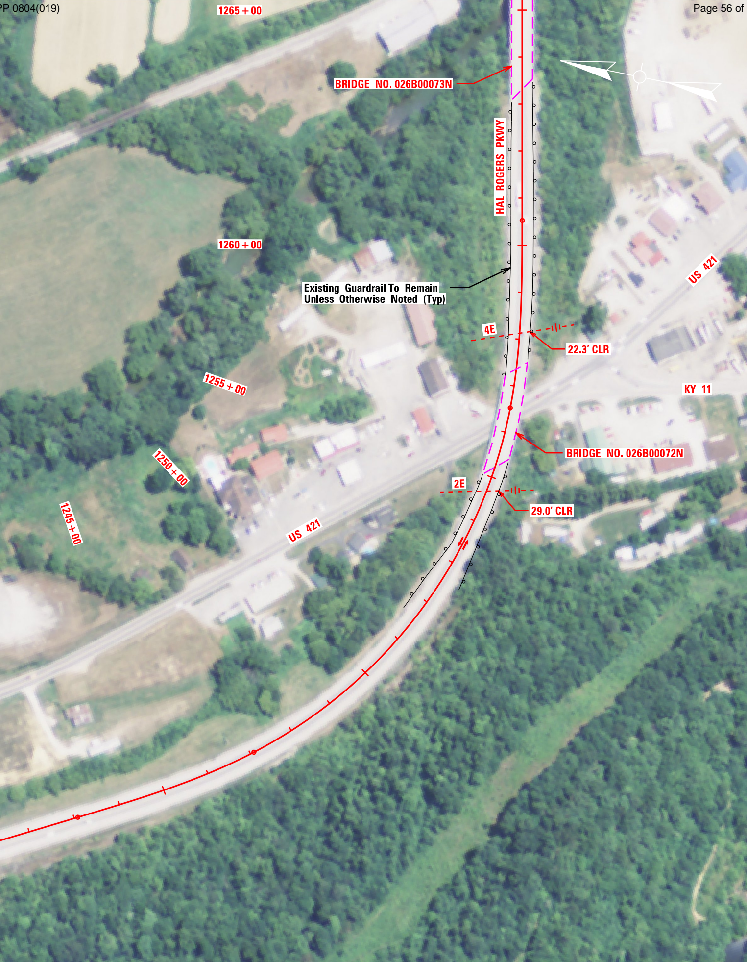
Hal Rogers Parkway Rehab Plan - Scale 1" = 200' - Sheet 6 of 44 - Sta 1245+00 to Sta 1265+00
