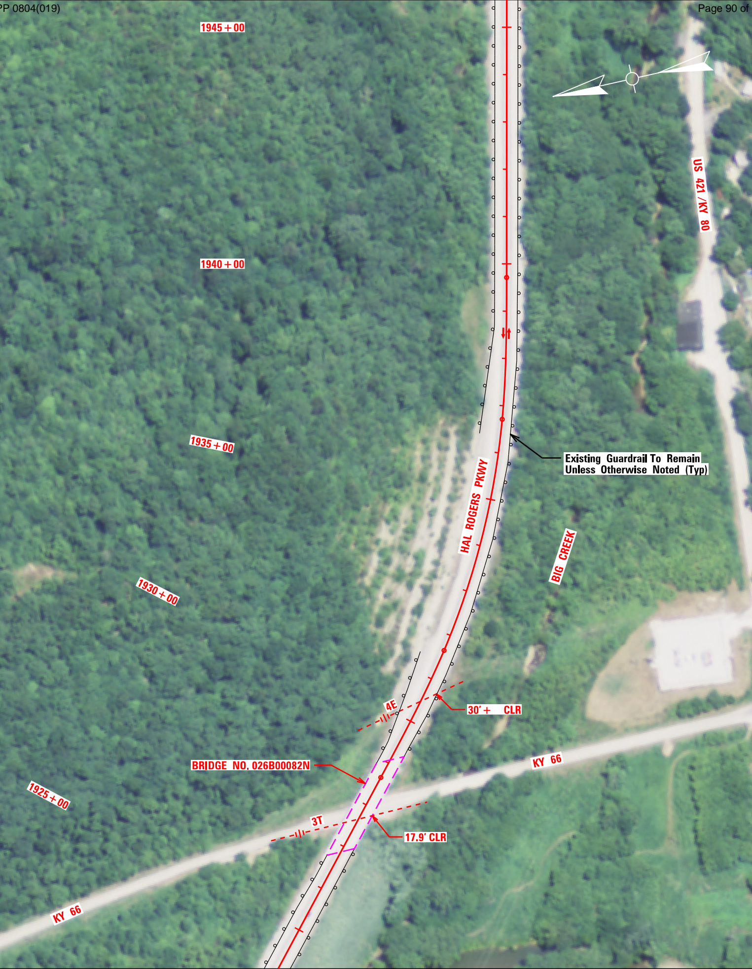
Hal Rogers Parkway Rehab Plan - Scale 1" = 200' - Sheet 40 of 44 - Sta 1925+00 to Sta 1945+00
