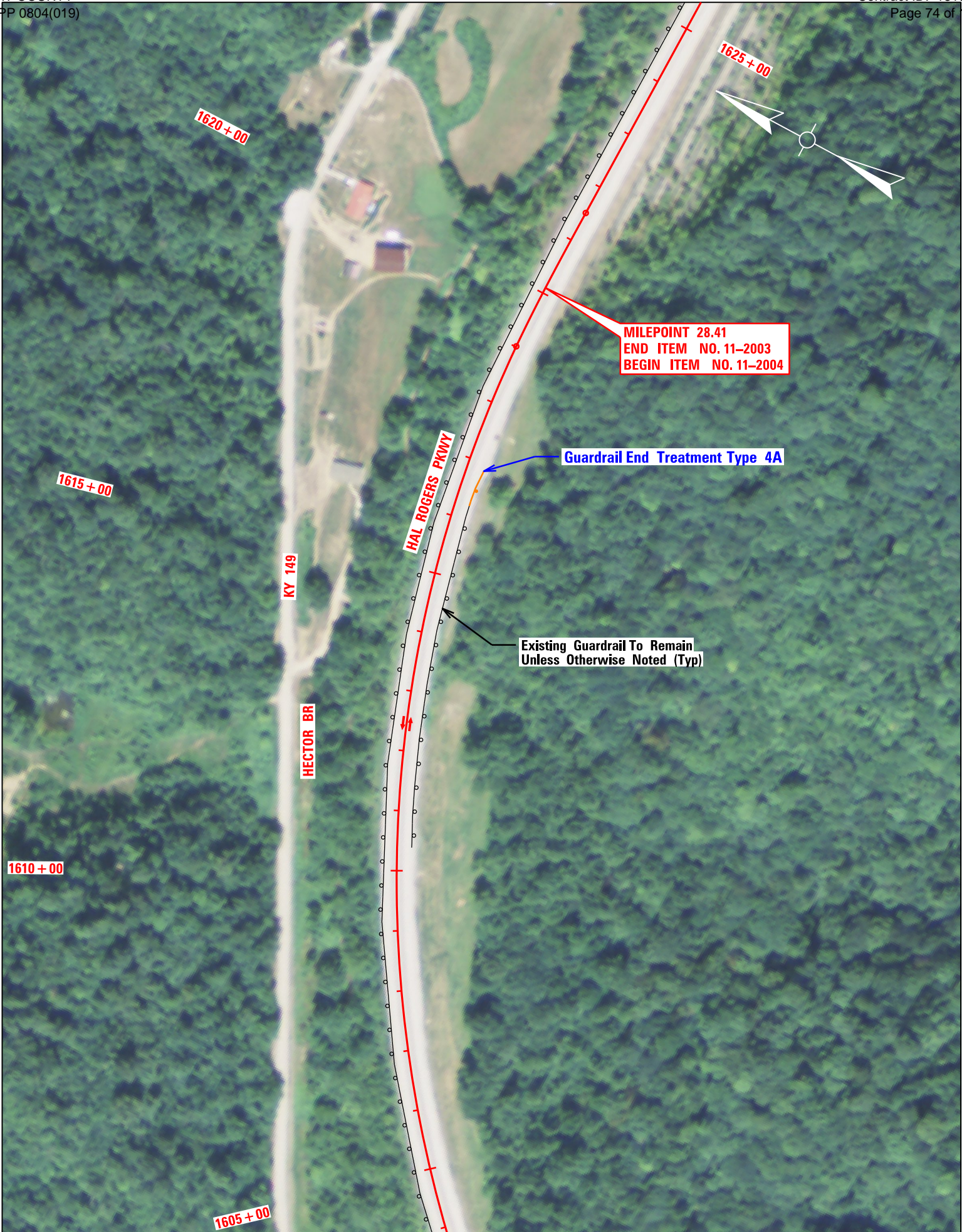
Hal Rogers Parkway Rehab Plan - Scale 1" = 200' - Sheet 24 of 44 - Sta 1605+00 to Sta 1625+00
