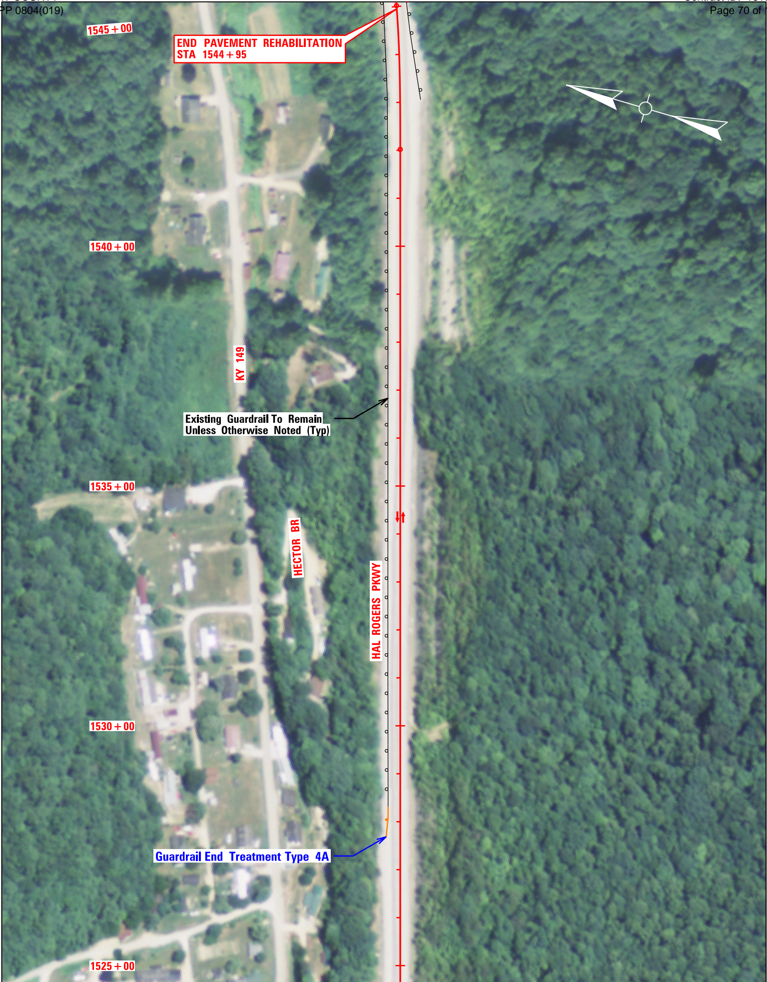
Hal Rogers Parkway Rehab Plan - Scale 1" = 200' - Sheet 20 of 44 - Sta 1525+00 to Sta 1545+00
