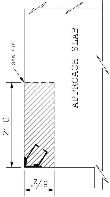
REMOVE X-HATCHED AREA OF CONCRETE AND ALL ARMORED EDGE MATERIAL.
