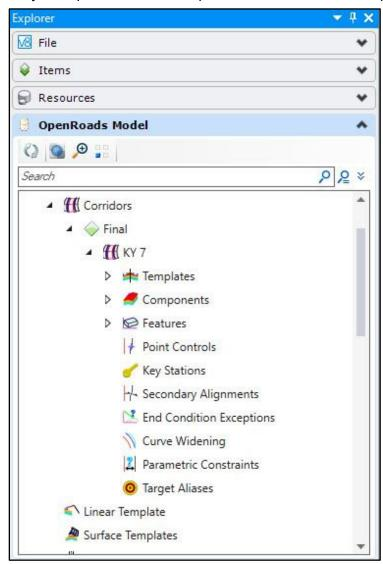
Within the Corridor, the designer can review the templates that were used, what components are associated to the templates, what point controls and end condition exceptions were used, etc. Terrain Model, Superelevation, Civil Cell, Linear Geometry and Alignment information can also be reviewed in this manner
