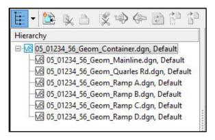
By referencing the individual geometry files, the designer can attach the Container File to other working files and have access to the civil data in each file. This will not only make it easier on the downstream user to understand the relationship of each file and thus each civil object but will make it easier for the designer to use them when creating other design elements. More information on the naming scheme of Container Files and the folder structure can be found in the current CADD Policy.
