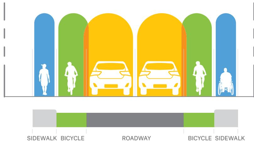
**Figure 3.13** Fully-shared bicycle, e-bicycle, e-scooter, and motor vehicle accommodations.
