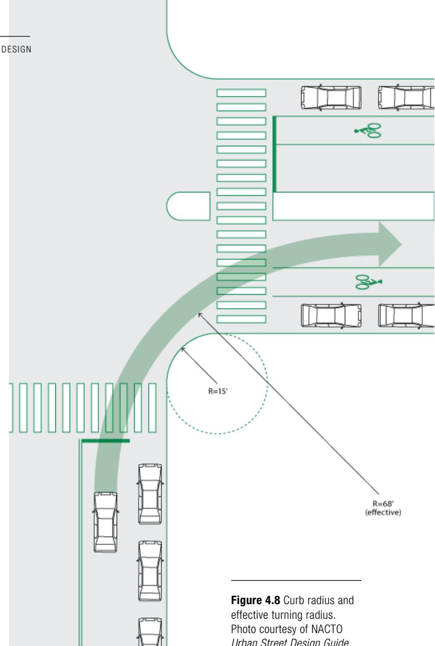
**Figure 4.8** Curb radius and effective turning radius.
