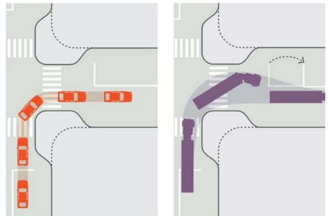
**Figure 4.5** Design (left) and control vehicle (right) turning radii.
