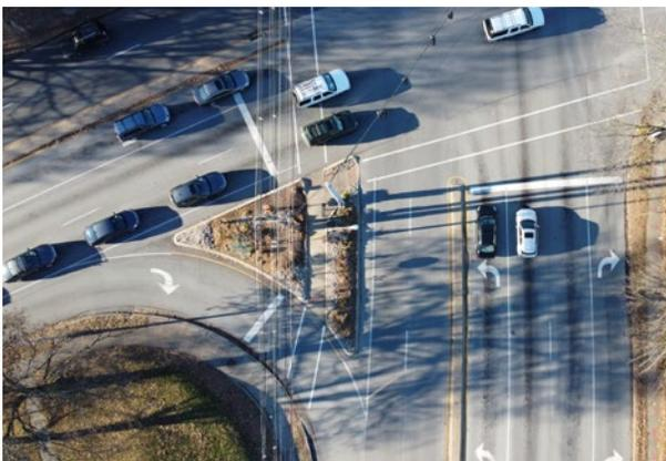
**Figure 4.10** Example of an intersection corner curb extension in Paducah, KY.
