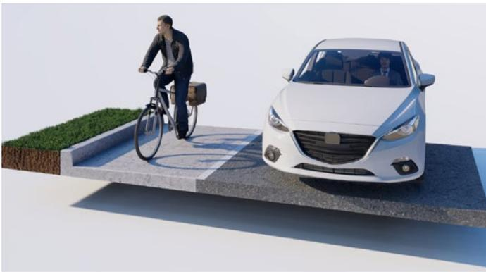
Where a gutter is present in the bicycle lane and does not span the full lane width, a minimum usable width of 3 feet and a preferred width of 4 feet measured from the longitudinal joint between the gutter and bicycle lane to the center of the lane pavement marking line is recommended.
