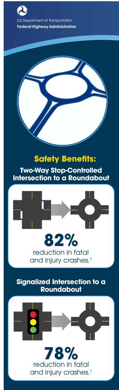
**Figure 6.13** Roundabout Proven Safety Countermeasure.
