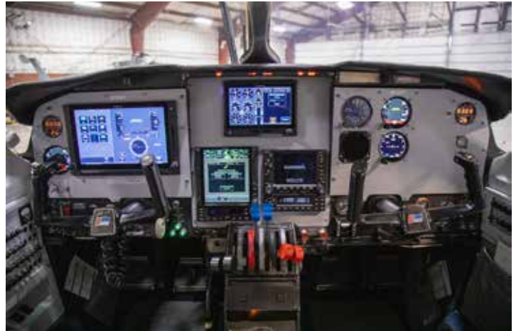
Avionics upgrade in state Piper Navajo Chieftain includes a G600 PFD, GI 275 back-up indicator, Garmin engine monitor, G750 TXI, and a S-Tec 3100 autopilot
