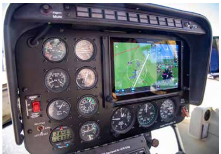
Avionics upgrade in both state helicopters (Bell 206) includes a Helisys autopilot, G500 PFD, and a G650 TXI
