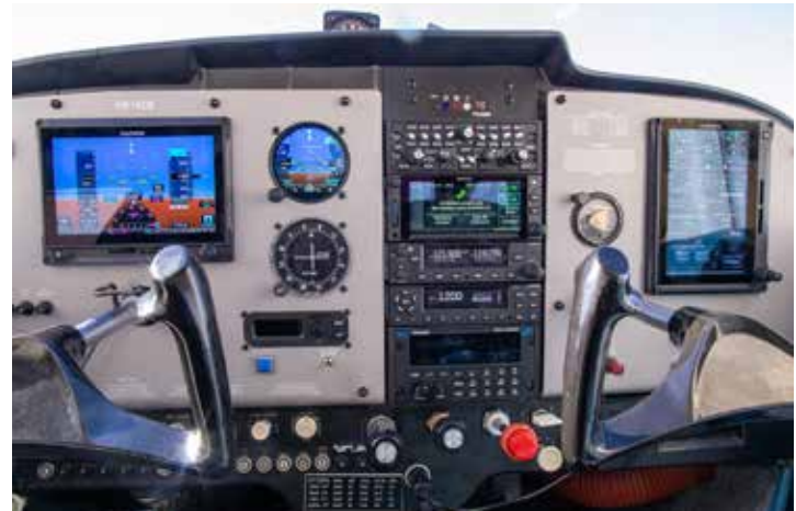
Avionics upgrade in the state aircraft Cessna 172 includes a G500 PFD, G275 back-up indicator, Garmin 650 TXI, G500 engine monitor & moving map display, and a Bendix King TruTrak autopilot
