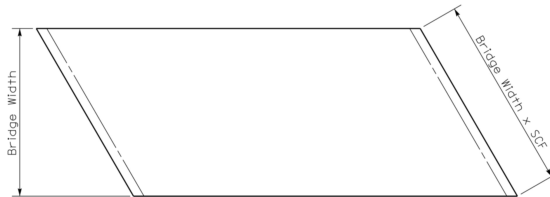
PLAN OF SUPERSTRUCTURE SLAB
