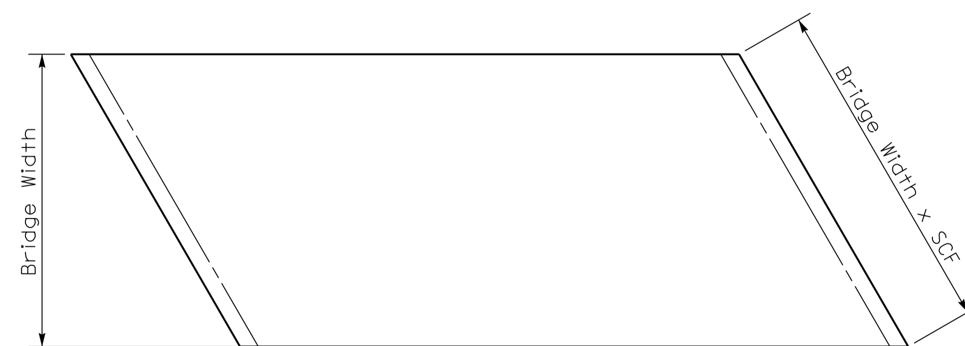
PLAN OF SUPERSTRUCTURE SLAB
