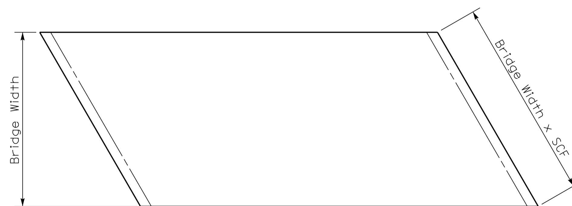
PLAN OF SUPERSTRUCTURE SLAB
