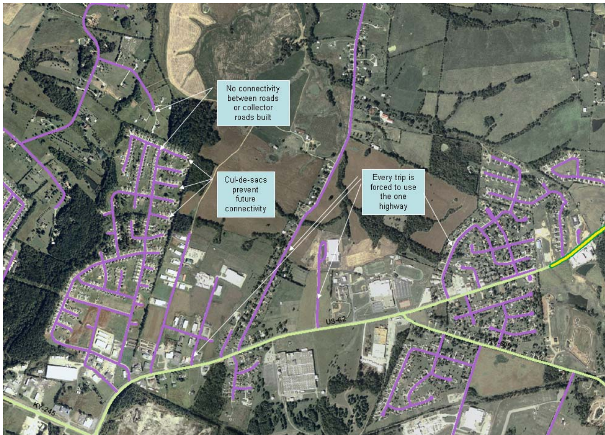
Figure 6: Examples of the lack of roadway interconnection
