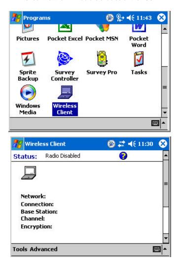
To enable the radio, select the "Enable Radio" option from the Tool menu.
