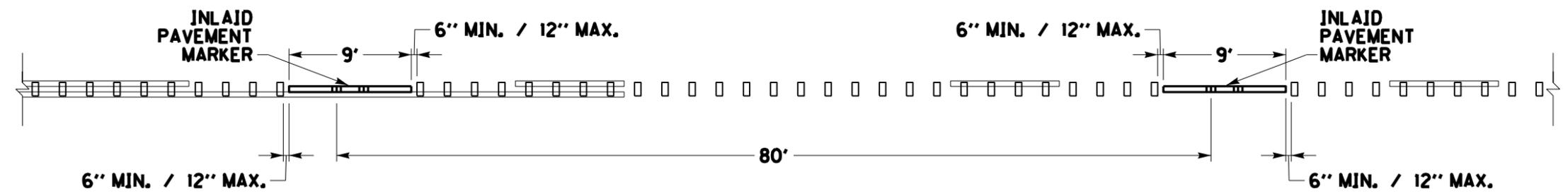
DETAIL FOR CENTERLINE RUMBLE STRIPS WITH INLAID PAVEMENT MARKERS
