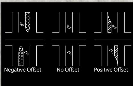
Removing left turning vehicles by using a left-turn lane can provide substantial safety and operational improvements. However, it is often difficult for a
