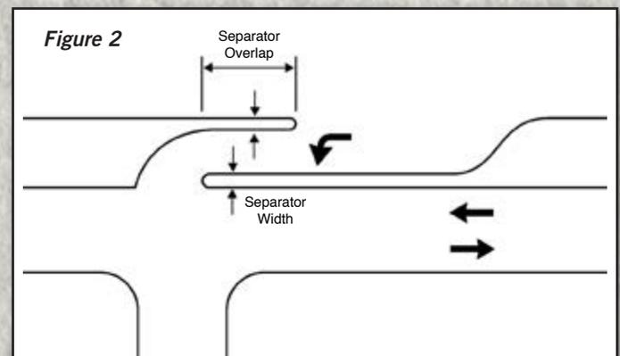
proximately 25 feet long. A median 18 feet wide is normally needed to allow for a raised concrete three-foot wide separator on each side and a 12-foot turning lane. In cases where space is limited, the width of separator overlaps may be reduced. (See Figure 2.)
