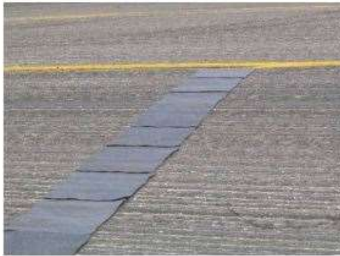
Figure 19. ASTM D 2995 Pads Used to Evaluate Transverse Application Uniformity
