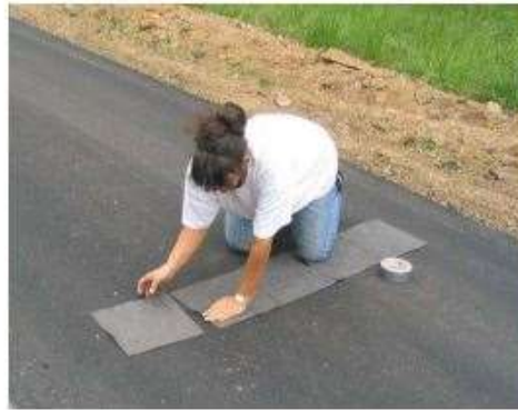
Figure 20. Placing Pads for ASTM D 2995
