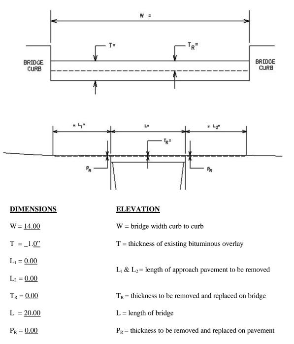
Notes: 1. The Engineer will determine lengths  $L_1 \& L_2$  by using a transition rate of 100 ft/inch of thickness.
