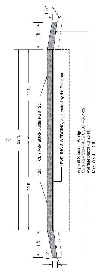
Wedge drop-offs greater than 1 inch with DGA as directed by the Engineer. \* 1" Maximum Drop-off Where Existing Site Conditions Permit
