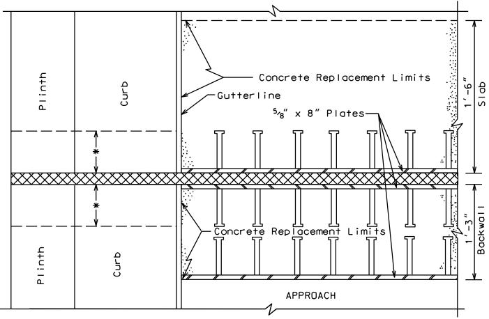
\* Remove and replace curb/plinth as directed by the Engineer to match proposed Expansion Joints (Incidental to "Expansion Joint Replacement").
