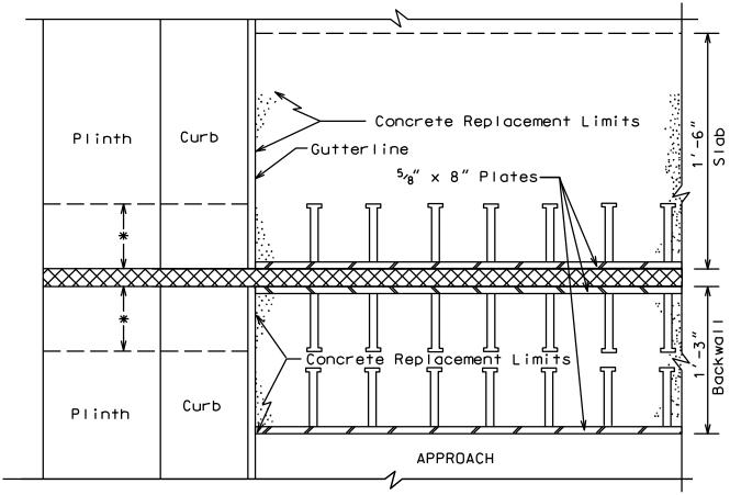
\* Remove and replace curb/plinth as directed by the Engineer to match proposed Expansion Joints (Incidental to "Expansion Joint Replacement").
