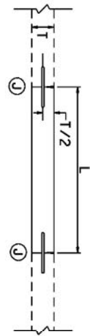
SECTION AAAA JOINT REPLACEMENT
