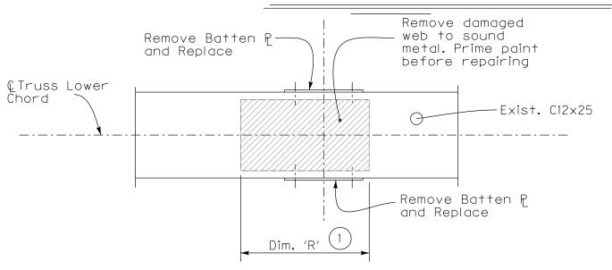
Note: field measure after removing deterioration and use dim 'R' to size repair P below.
