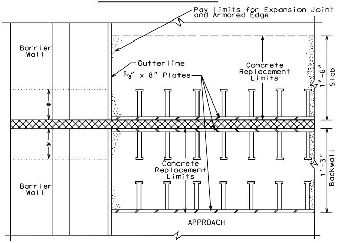
\* Remove and replace barrier wall as directed by the Engineer to match proposed Expansion Joints (Incidental to "Expansion Joint Replacement").
