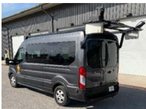
KYTC's automated pavement data collection equipment
