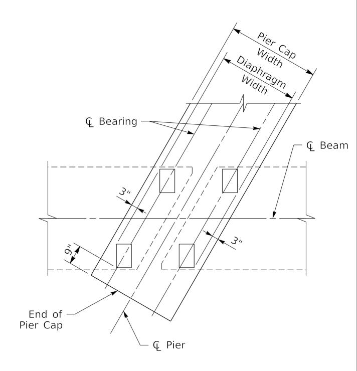
Dimensions shown to pad edges are minimums. Take care to ensure beams are not overhanging pier caps excessively when single pads are used under beams with large bottom flange widths. The Division of Structural Design reserves the right to require larger dimensions than those shown
