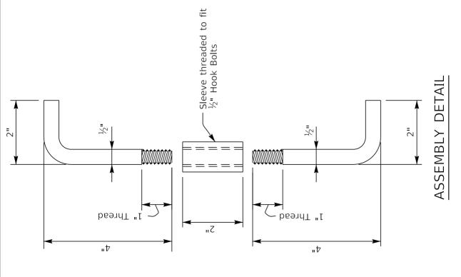
Hook Bolt Assembly requires a minimum tensile strength of 4 kips when assembled as a unit. Both Hook Bolts and Sleeve are made of steel and meet the requirements of ASTM A307.
