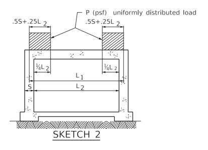
On multiple barrel culverts :  $L_1$  = Distance center to center of Exterior Walls  $L_2$  = Distance from inside of Exterior Wall to inside of Exterior Wall
