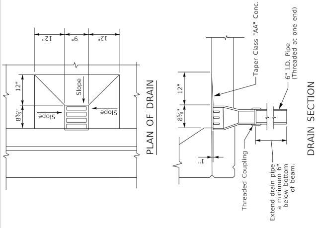
Drain Pipe and Fittings are 6" I.D., 0.25" minimum wall thickness, wound with fiberglass epoxy resin formulation with ultraviolet inhibitors. Supply the pipe pigmented to match the final color of the structure.
