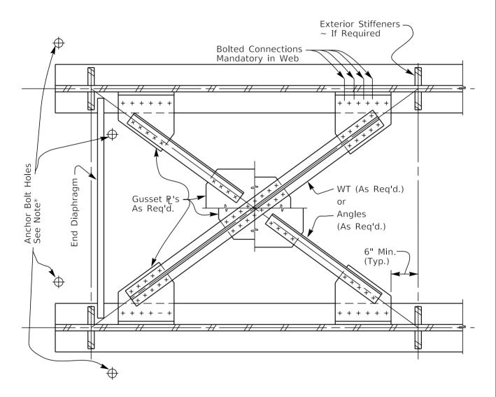
Fasteners shown are for illustration only. WT's may be welded to Gussets
