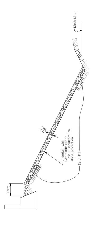
Include bid item for crushed aggregate slope protection quantities in plans.
