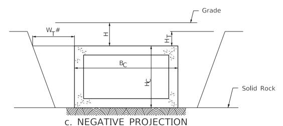
$\mbox{\# If } W_{\mbox{\footnotesize{T}}}\mbox{exceeds 6' consider the culvert to be in a Positive Projection}$
