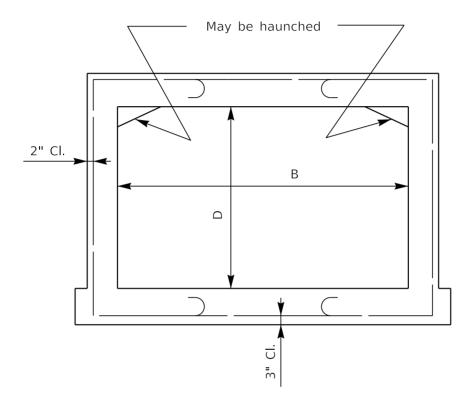
Reinforcement for Corners may be hooked rather than continuous across slab to facilitate placement.
