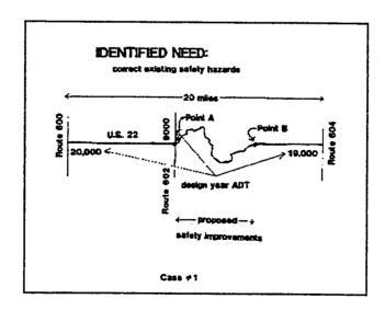
U.S. 22 is a rural two lane facility without access control. A number of high accident locations have been identified, and the need for the project is to correct site specific geometric deficiencies between point A (Route 602) and point B (no intersecting roadway).
