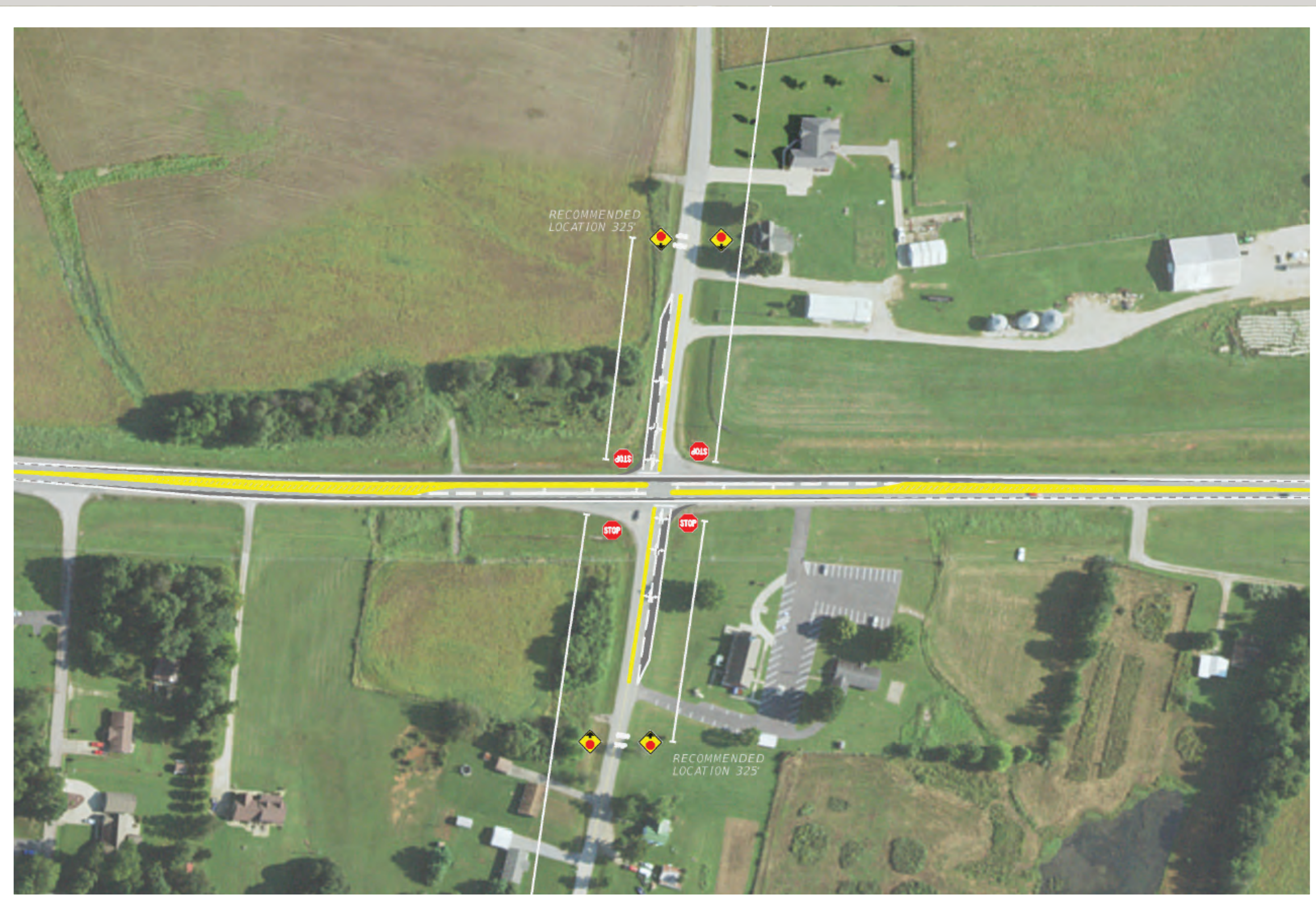
LEFT-TURN LANES ON KY 210 & NORTHBOUND KY 470. STOP AHEAD SIGNAGE & PAVEMENT MARKINGS.
